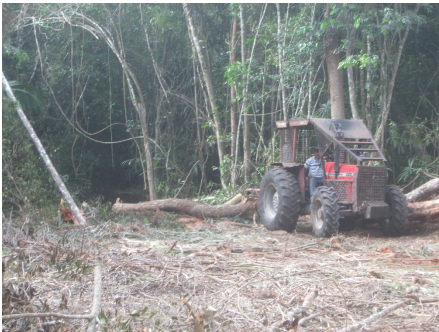
Forestry practices in the region are already low impact. Here a modified tractor-skidder hauls a log to a landing area.
