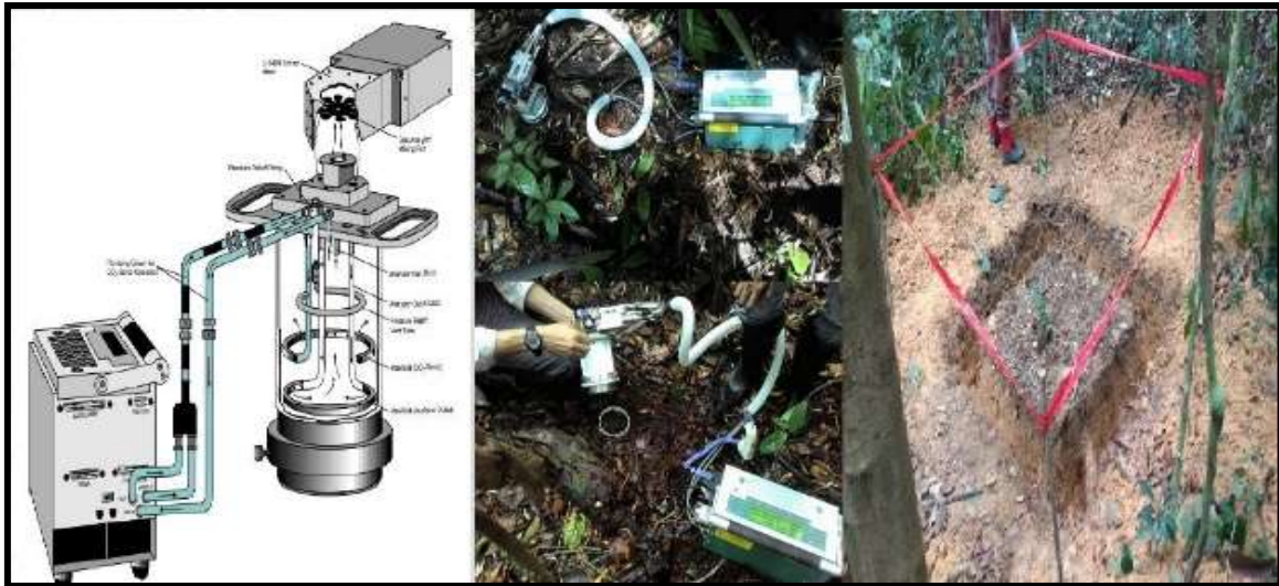
Fig. 4: CO 2 efflux from soils was measured using a LiCOR6400XT (portable photosynthesis system)(left pic) configured with the soil respiration chamber(middle pic) using trenching method (right pic)
