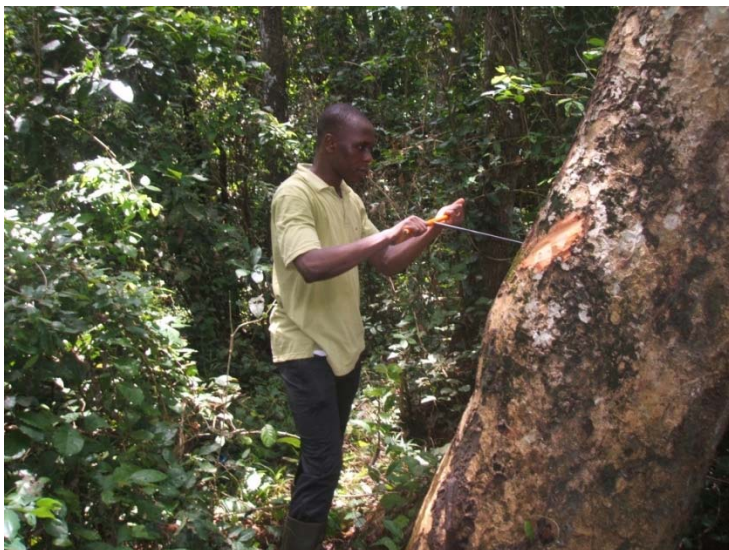
Collection of wood samples using an increment borer in a tropical forest in Benin for basic wood density measurement
